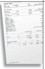
The DL22 F&B automatically calculates results using predefined units. Depending on the method selected, METTLER TOLEDO has predefined the most common calculations using the appropriate units. The results are stored and can be printed out as a clearly structured report via the compact METTLER TOLEDO RS-P42 laboratory printer.
