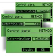
The DL22 F&B is a specialized titrator for the food and drink industry. It incorporates the methods most widely employed in these industries and uses predefined parameters. This makes work considerably easier. Three predefined options are available for selecting the control parameters for the titrations.
