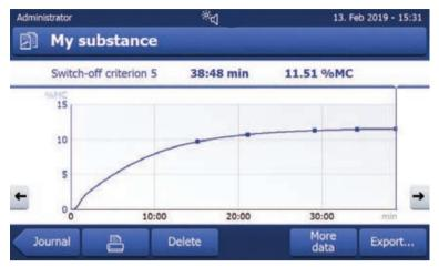
In the graphical visualization of the test process, the details about the different SOC (time and % MC at the point of reaching) can be accessed:
