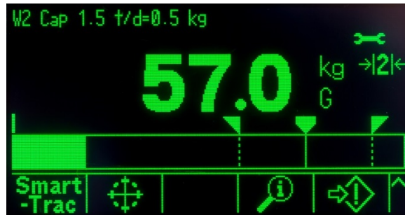
Figure 1-11: Small Material Transfer SmartTrac Enabled
