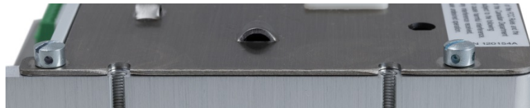
Figure 2-127: Sealing Screws Installed
