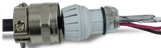
Figure 2-71: Inner Shield Unbraided and Folded Back over Grommet
