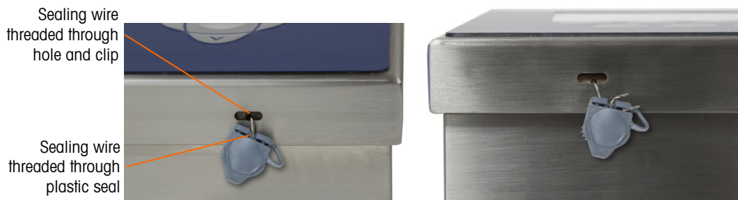
Figure 2-130: Harsh Enclosure Seal Threaded and Ready to be Closed – Standard Orientation (left) and with Panel Reversed (right)
