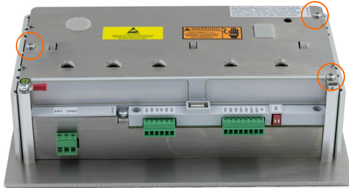
Figure 2-1: Opening the Panel-Mount Enclosure
