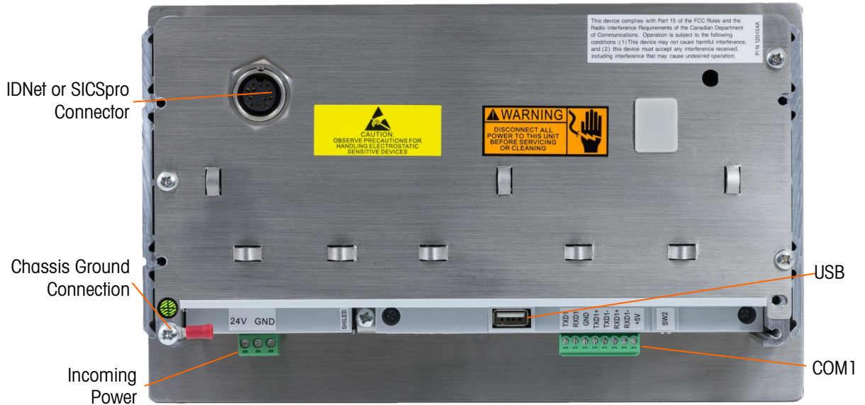
Figure 2-27: Panel Mount Enclosure Connections, including IDNet Scale Interface
