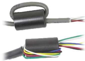
Figure 2-20: Installing the Ferrite Cores
