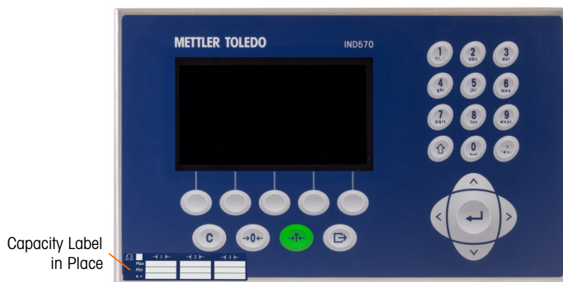
Figure 2-125: Capacity Label Installed
