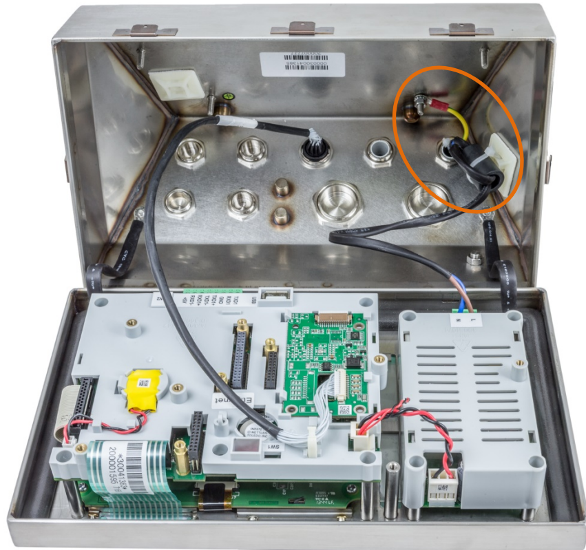
Figure 2-17: Front Panel and Load Cell Connection Reversed
