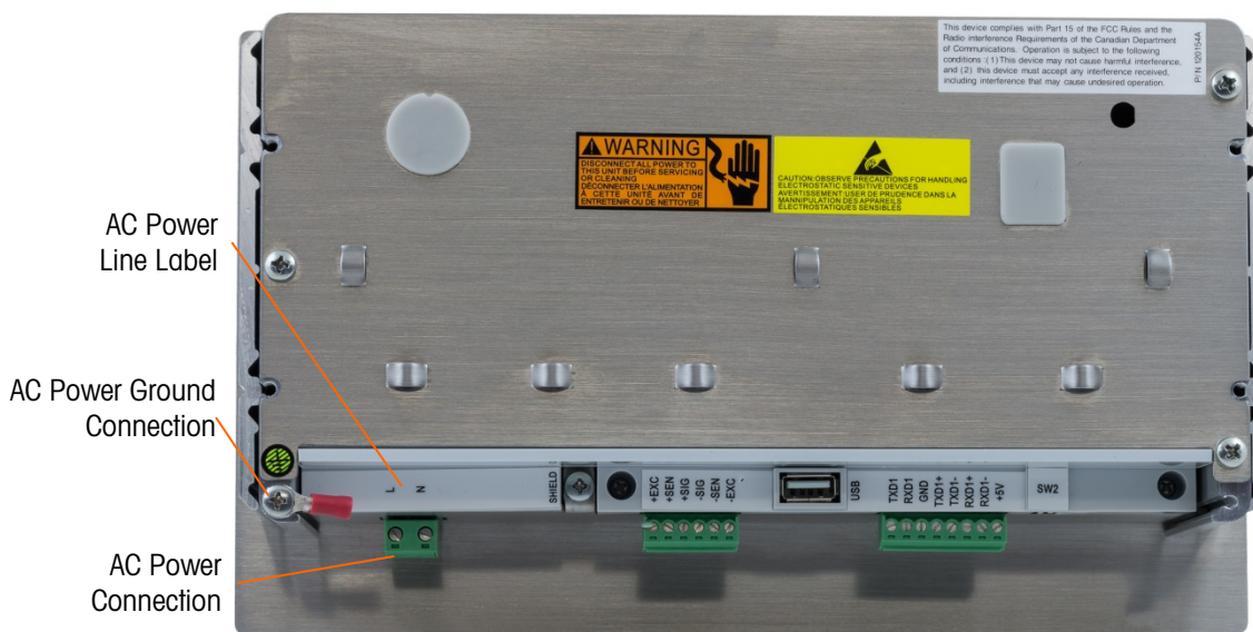
Figure 2-29: AC Power Connection on Panel Mount
