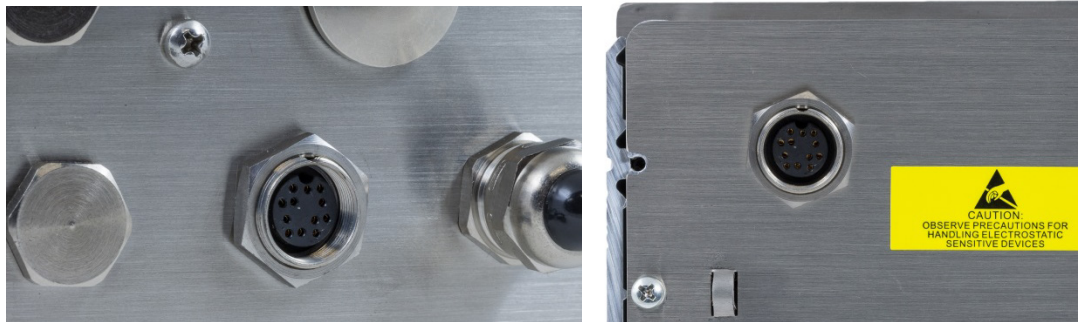
Figure 2-32: IDNet Connector Location on the Harsh (left) and Panel (right) Enclosures
