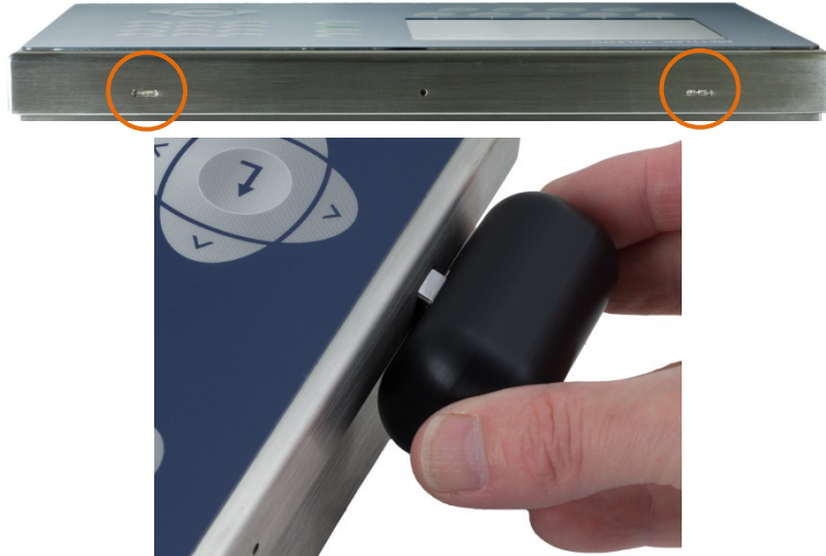
Figure 2-2: Opening the Harsh Enclosure, Preferred Method
