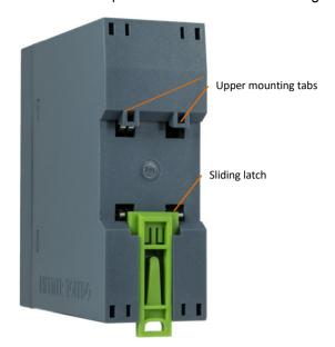
To mount the ACT350POWERCELL on a rail, open this latch by pulling down on it, then position the transmitter so that its upper tabs rest on the DIN rail.
